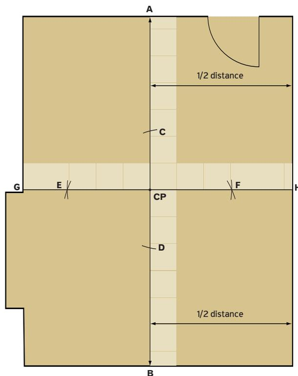
Figure 1 Setting out with loose lay tiles
