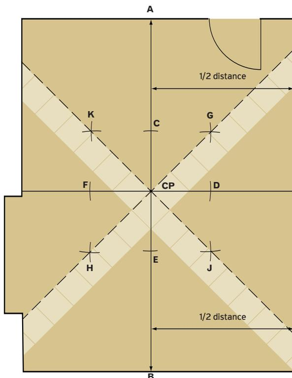
Figure 2 Diagonal setting out with loose lay tiles
